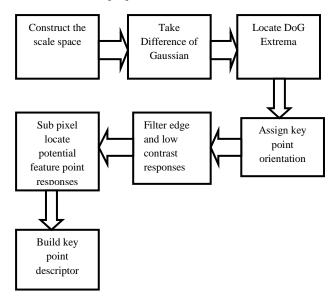
Fig. 2. Design flow for SIFT Algorithm
