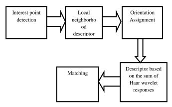
Fig. 3. Design flow for SURF Algorithm
