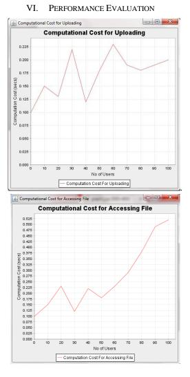
Figure 4: i) Computational cost achieved at uploading ii) Computational cost accessing file.
