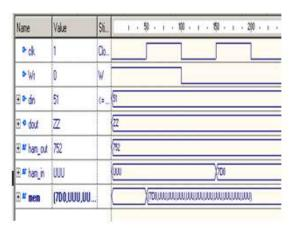
Figure.3. Simulation waveform for fault-tolerant : system using Hamming code with double faults in memory
