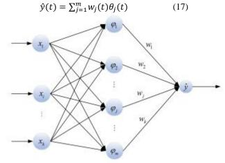
Figure 4. The structure of RBFNN.
