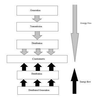
Figure 1.1 New industrial conception of the electrical energy supply
