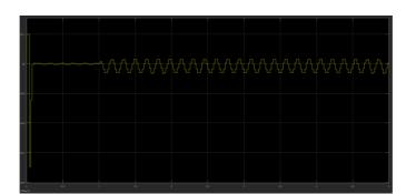
Fig4.9 Plot of Frequency in Normal Mode and Islanded Mode of Operation
