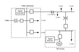
Figure 2.3: Distributed Generation power line Signalling Islanding Detection
