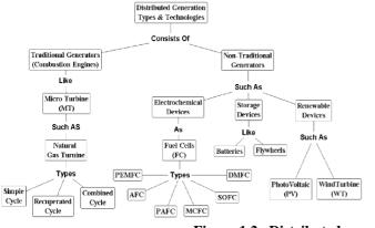
Figure 1.2. Distributed generation types and technologies
