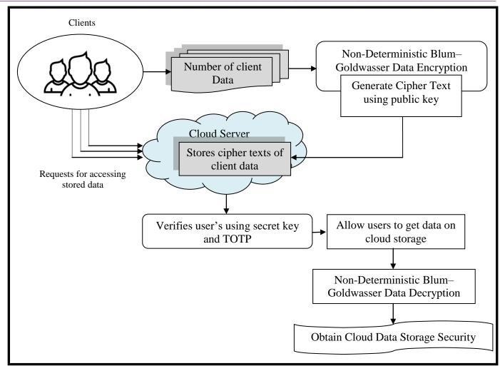
Figure 1 Architecture Diagram of SSNBTOPC Technique for Cloud Data Storage Security
