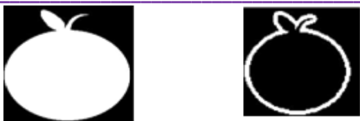
Figure 2: (a) Original Image (b) Skeletonized image
