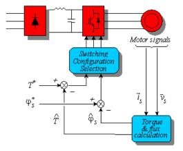
Fig. 11. Block diagram of DTC
