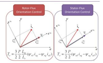
Fig. 6 Vector diagram for Flux oriented control method
