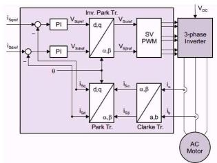
Fig. 8 Block diagram of Rotor Flux Oriented Control method
