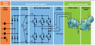
Fig.1 Block Diagram of Electric Motor Drive System
