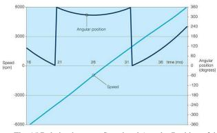
Fig. 15 Relation between Speed and Angular Position of the Induction Motor Drive with FOC and DTC.
