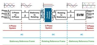
Fig. 3 Concept of Space Vector Modulation
