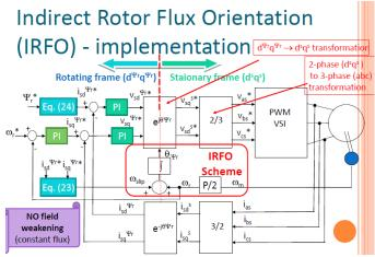
Fig. 10 Block diagram of Indirect Rotor Flux Oriented Control method
