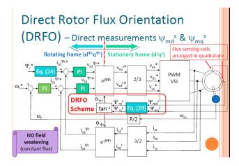
Fig. 9 Block diagram of Direct Rotor Flux Oriented Control method
