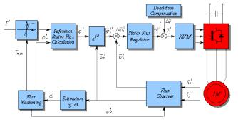
Fig. 7 Block diagram of Stator Flux Oriented Control method
