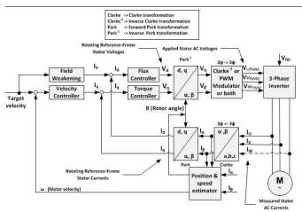
Fig. 4 Field Oriented Control of Induction Motor
