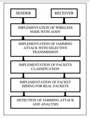
Fig. 2: Block Diagram of the proposed system.
