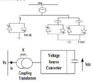
Figure 2 Diagrams of SVC and STATCOM [8]
