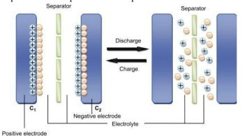
Figure 4 Super Capacitor Working
