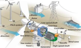
Figure 1 Wind turbine Working Principle
