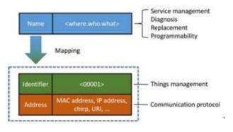
Fig. 5. Naming Mechanism inEdgeOS.
