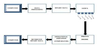
Figure 3: Block diagram of a VLC system
