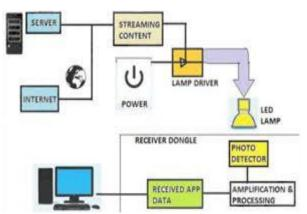
Figure 1: Working of LED in Li-Fi technology
