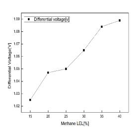
Figure 7. The response Characteristics of Sensor by Methane Gas Concentration (Based Voltage)
