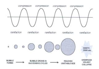
Figure 2. Growth mechanism of the ultrasonic method
