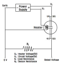
Figure 4. A sensing circuit for a semiconductor gas sensor
