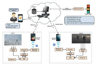
Fig 2.5.1: Architecture of Traffic Congestion & Monitoring System
