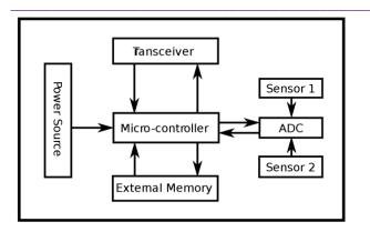
Fig 3.1.1. Architecture of wireless sensor node.
