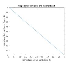
Figure 6. Slope between bands for noise free image
