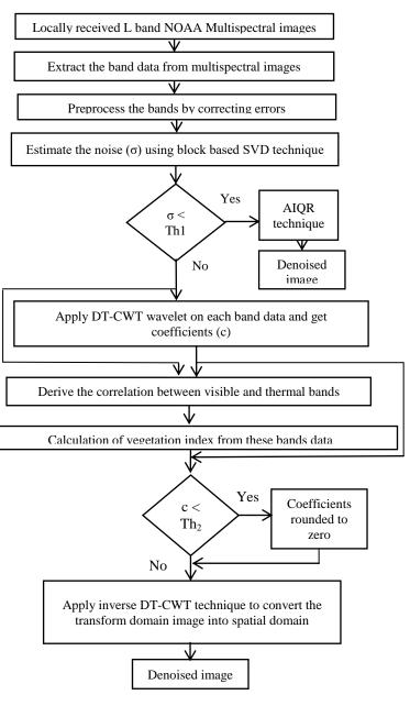
Figure 5. Flow chart of the proposed denoising technique for NOAA data
