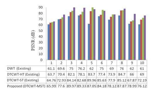
Figure 10. Comparison of performance (PSNR) of frequency domain denoising techniques for NOAA images
