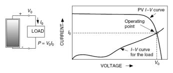
E. Module supplying power to a Resistive load
