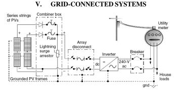
• Principal components in a grid-connected PV system using a single inverter
