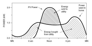
• During the day, excess power from the array is sold to the utility; at night, the deficit is purchased from the utility - a single electric meter runs in both directions.
