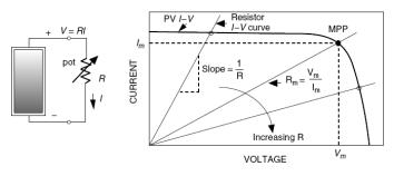
• As resistance changes, the operating point moves around on the I – V curve
