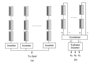
• Large grid-connected systems may use an individual inverter for each string (a) or may incorporate a large, central inverter system to provide three-phase power (b)
