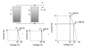
Each module is rated at 180 W, but the parallel combination yields only 330 W at the maximum power point.
