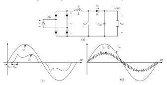
Fig. 2. Boost-type SMR: (a) circuit; (b) sketched key waveforms for low-frequency switching; (c) sketched waveforms for high-frequency switching
