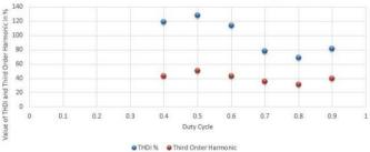
Fig. 6 Variation of THD<sub>i</sub> and 3<sup>rd</sup> order harmonic with respect to duty cycle.
