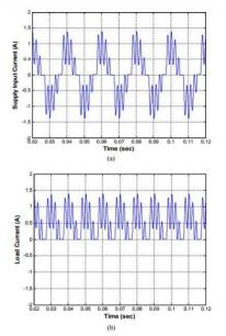
Fig. 8 Passive Wave Shaping method Supply input current and Load Current.
