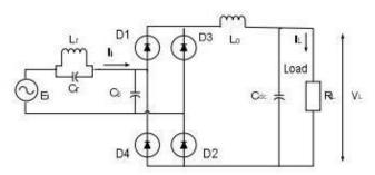
Fig. 7 Passive Wave Shaping Filter
