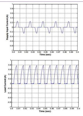
Fig. 3 VSF Supply Input Current and Load Current
