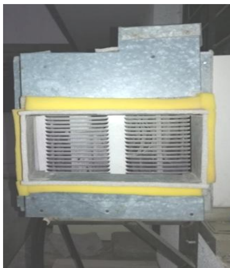
Figure 2. Pre Cooler Area of Window Air-Conditioner with Duct and Passage for Air Pre-Cooler
