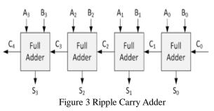
Sum out  $S_0$  and carry out  $C_{out}$  of the Full Adder 1 is valid only after the propagation delay of Full Adder 1. In the same way, sum out  $S_3$  of the Full Adder 4 is valid only after the joint propagation delays of Full Adder 1 to Full Adder 4. In simple words, the final result of the ripple carry adder is valid only after the joint propagation delays of all full adder circuits inside it. The block diagram is shown in figure 3.
