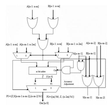
Figure 1 Architecture of static segment adder (SSA)
