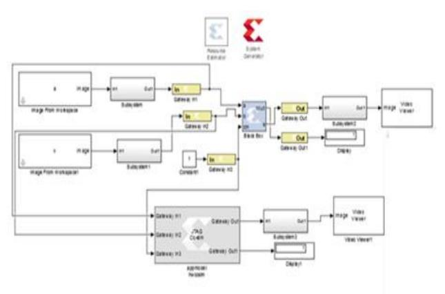
Figure 9 Xilinx Block for Hardware Implementation
