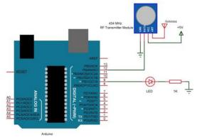
Figure 12. RF Trasmitter interfacing with Arduino
