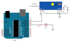
Figure 14. RF Receiver interfacing with Arduino
