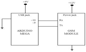
Figure 10. Interfacing of GSM module with Arduino.
