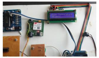
Figure 18. Diplaying Body Temperature of the patient using LCD.
