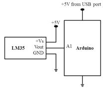
Figure 6. Interfacing of LM35 with Arduino.
