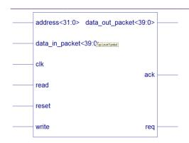
Fig.6: RTL Schematic of OLSR Protocol under black hole attack
