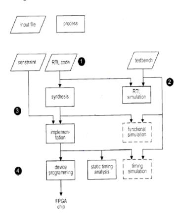
Fig. 5: FPGA XILINX process
