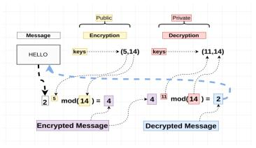
Figure 2.2 Encryption and decryption of RSA
