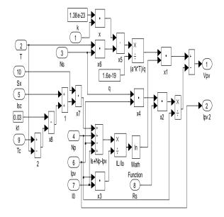
Figure 4. PV Array Matlab/Simulink functional model.
