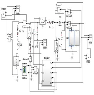
Figure 6: The general Matlab/Simulink model of PV array and Li-Ion battery powered LED lighting system.
