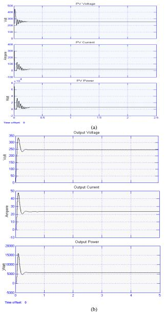
Figure 9. (a) PV voltage, current and power, (b) output voltage current and power simulation results without battery and PID controller
