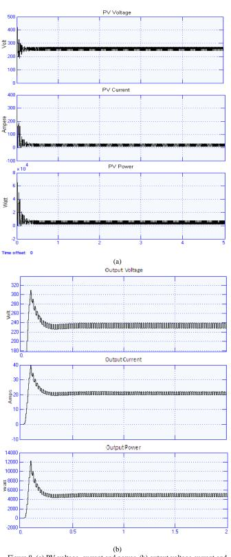
Figure 8. (a) PV voltage, current and power, (b) output voltage current and power simulation results for SOC 50%.
