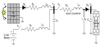
Figure 2. Test system PV and battery powered LED lighting system.
