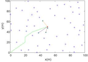
Figure 9. Target tracking in WSN using Particle Filter.
