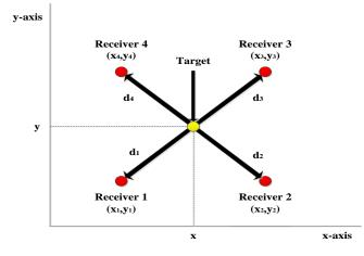
Figure 5. Two-dimension schematic indoor floor space geometry of human and four recievers.
