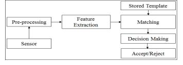
Figure 1. Block diagram of Biometric system [2]
