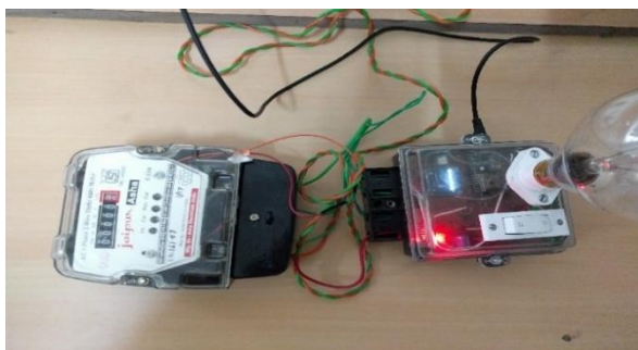
Fig. 4 Experimental setup of IoT based smart energy meter in laboratory
