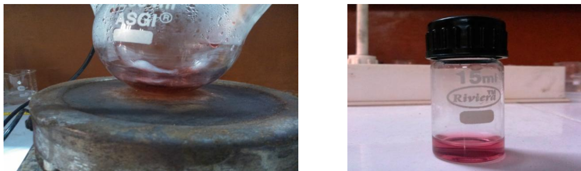
Fig.8: Formed gold nanoparticles using Green synthesis method
