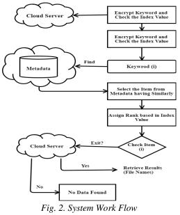
First of all encryption process is done. This is done by a hybrid algorithm. Here we use AES and RSA algorithm. The
