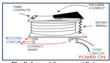
Fig. 8: Internal Structure of Relay
