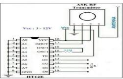
Fig. 14: Circuit diagram of RF transmitter
