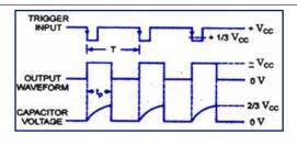
Fig. 11: Waveforms of Monostable multivibrator
