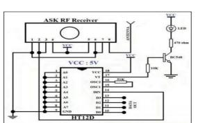
Fig. 16: Circuit diagram of RF receiver
