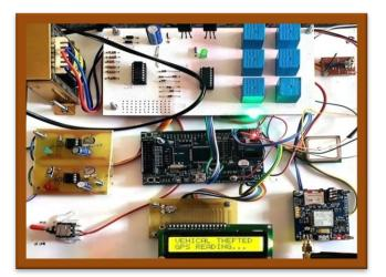
Fig. 22: Display of Vehicle theft detection
