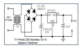
Fig. 5: Volts regulated power supply
