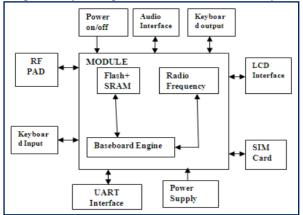
Fig. 17: GSM module structure
