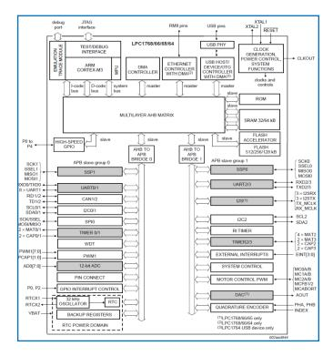
Fig. 2: Block diagram LPC 1768 ARM Cortex M-3
