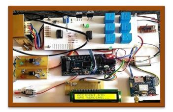
Fig. 20: Accident detection displays on LCD
