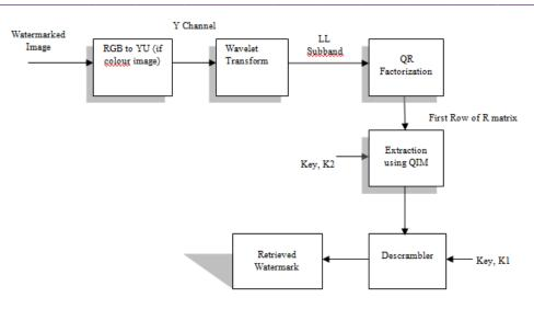
Figure 2: Block diagram of Extraction Scheme
