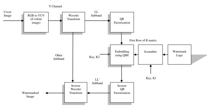
Figure 1: Block diagram of Embedding Scheme
