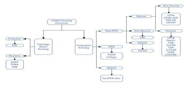
Figure 2: Routing Protocols in VANET [12]
