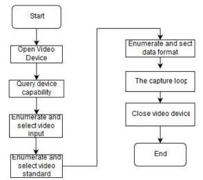
Fig. 7 The operation procedures of V4L2
