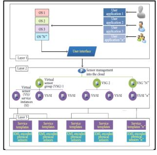
Figure 1: Layered structure for Sensor-Cloud
