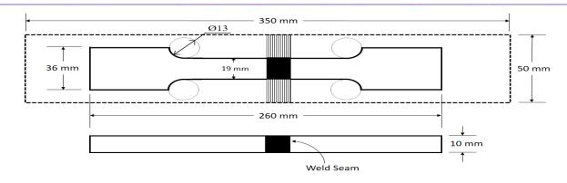
Figure 5 Tensile specimen
