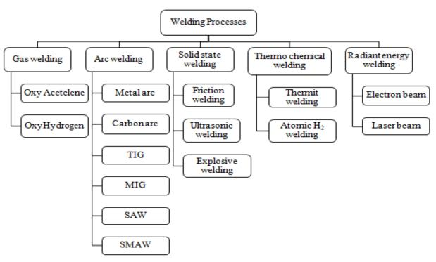
Figure 1 Classification of welding process
