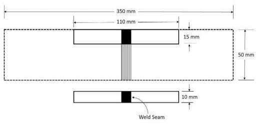
Figure 7 Hardness specimen
