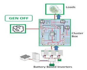
Fig. 6 Cluster Box Power Flow when Generator is OFF
