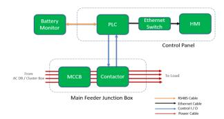
Fig. 9 Block Diagram of Load Shedding Panel H. Power Room
