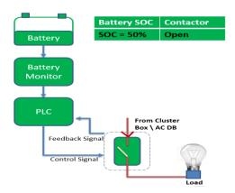
Fig. 11 Operation of Load Shedding Panel for Battery State of Charge (SOC) <50%
