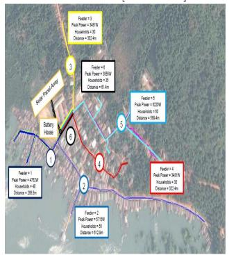
Fig.8 Distribution Network Table 6.3 Feeders Loss Calculation
