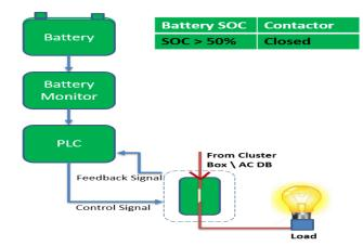
Fig. 10 Operation of Load Shedding Panel for Battery State of Charge (SOC) >50%
