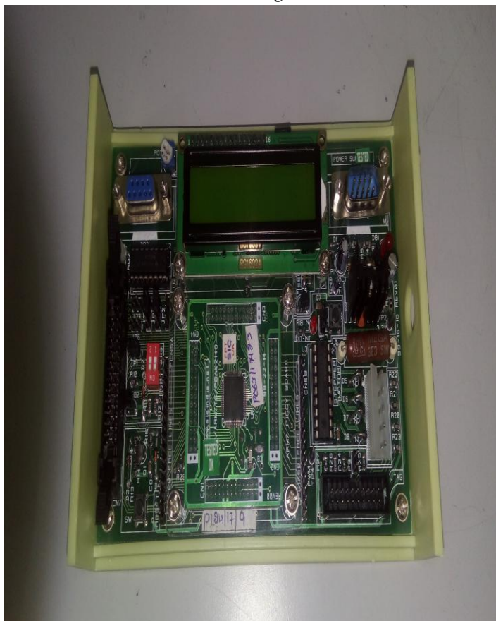
Fig.3 photographic view of the ARM-09 NXP LPC2148 Microcontroller board
