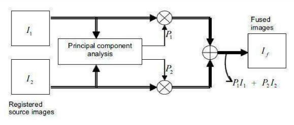
Figure 4 : Information Flow Diagram Of PCA
