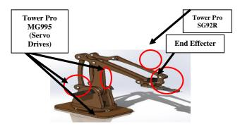
Fig 5: Solidworks View of Robot
