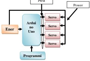
Fig 1: Block diagram of Robot
