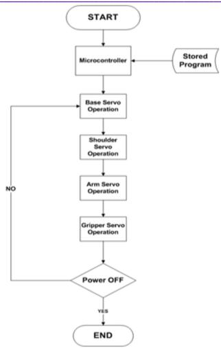
Fig 3: Flow Chart of Arduino Programme
