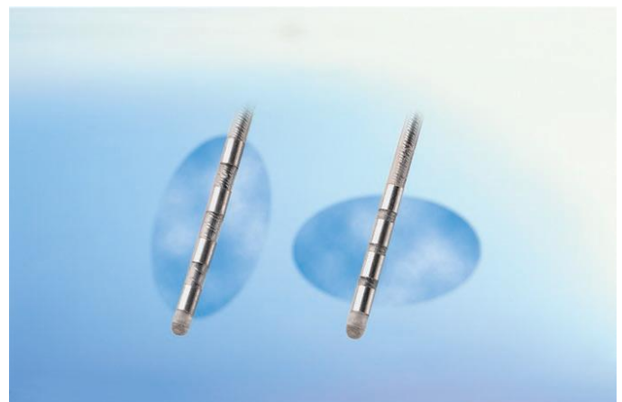
Figure 2 The quadripolar electrodes (leads) used for deep brain stimulation. (The contact is 1.5mm long and 1.27 mm diameter. The left microelectrode is Model 3387 and right model is 3389) Courtesy Medtronic, Inc.
