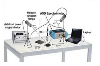
Figure 2. Setting and the internal structure of the ASD spectroradiometer [31]
