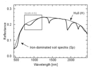
Figure 1. Spectral signature of iron oxide
