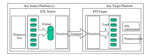
Figure 4. The ETL process
