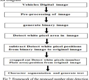
Fig.2. Framework of the proposed number plate detection approach.
