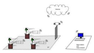
Figure 2. (Network star topology architecture) Distribution of the modules for a surface  $A_1$ .
