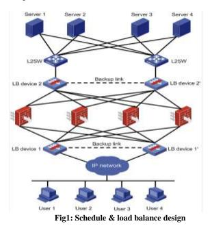
Let us take 4 servers (Server1, through Server4) are interconnected with two routers (L2SW1 & L2SW2), and 2 Load Balancing devices (LB Device2 and LB Device 2') are connected to two routers (L2SW1 & L2SW2). The 2 Load Balking devices connected to another 2 Load Balancing devices (LB Device 1 and LB Device1') through interconnected Fire walls for security purpose and connected through cloud to different users located geographically.
