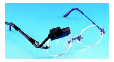
Fig 2: Eyeglass display with Holographic element.
