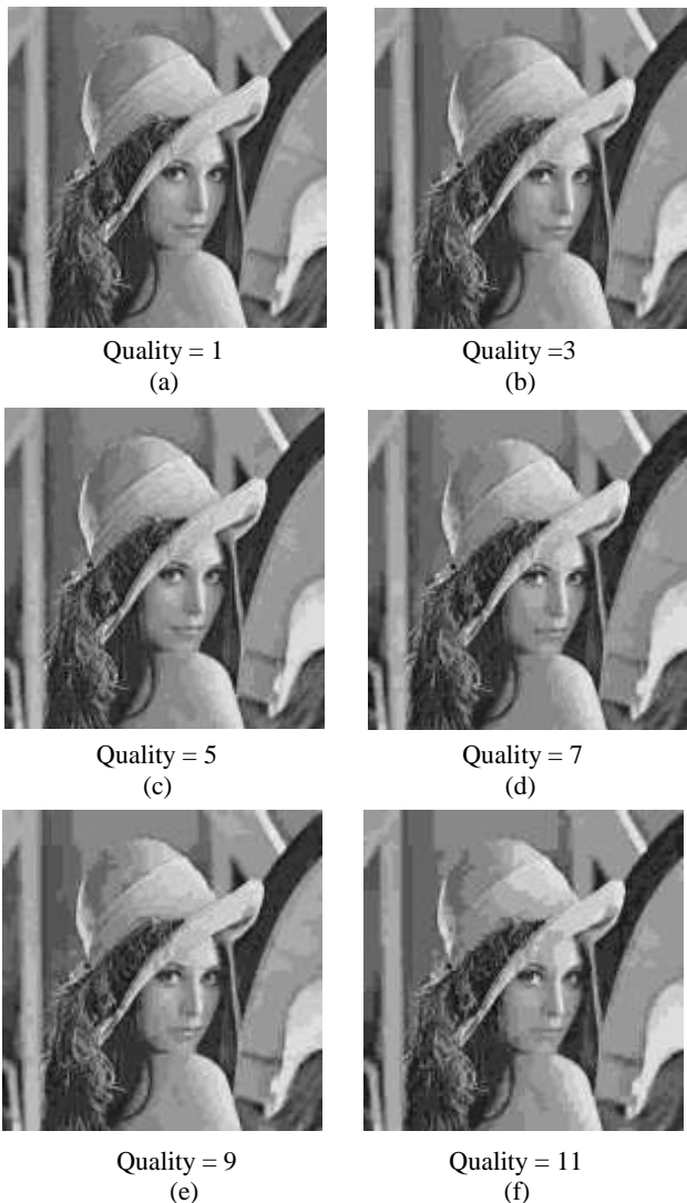
Fig. 5. Restoration Results of HLPC-DCTC for 'Lena' Image for Different Values of Quality (a) Quality = 1 (b) Quality = 3 (c) Quality = 5 (d) Quality = 7 (e) Quality = 9 (f) Quality = 11
