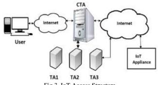
Fig.3 IoT Access Structure
