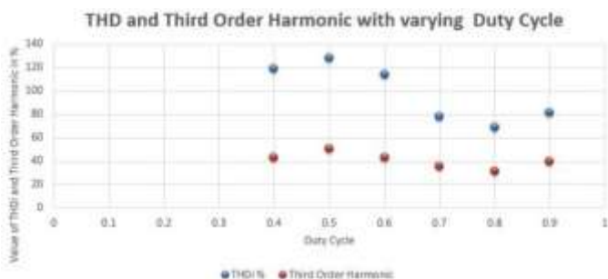
Fig. 6 Variation of THD i and 3 rd order harmonic with respect to duty cycle.
