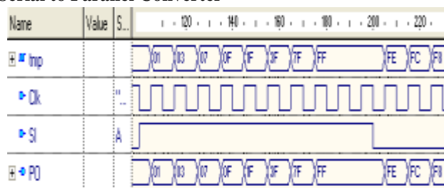
Fig 3.5 Simulation results of serial to parallel converter
