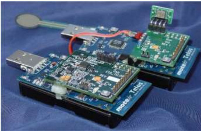
Figure 1: ActiS sensors with customized daughter boards [17].
